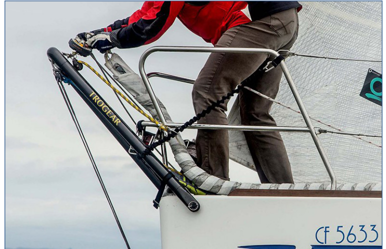
Fig 3: Bowsprit in upright position to attach a furler.
