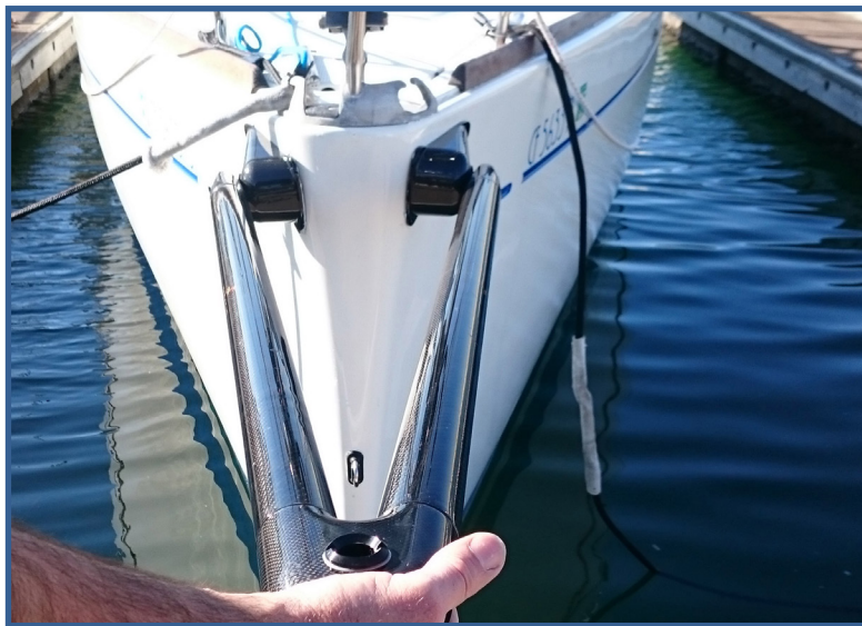
Fig. 1: Place bowsprit with mounts attached on the hull to determine location
