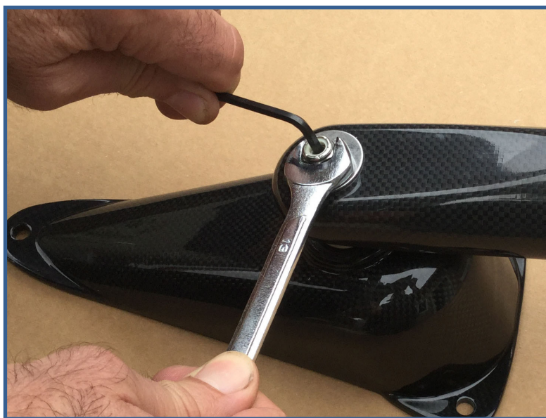
Fig. 2: Use allen wrench to prevent stud rotation
