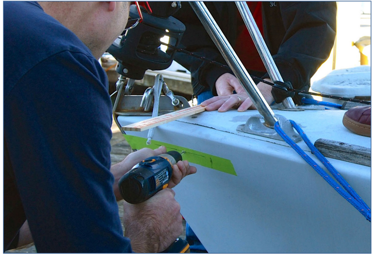
Fig 6: Drill a pilot hole first.
