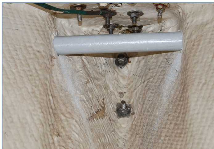
Fig. 2: Inside the hull showing the Hinge Tube installed
