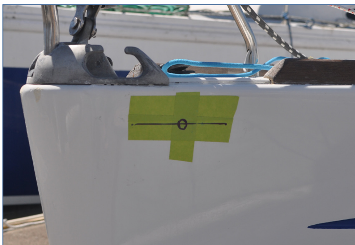
Fig 5: Using non-stretching line attached to the headstay, or other method as appropriate, check that the distances you marked are the same on each side of the boat.
