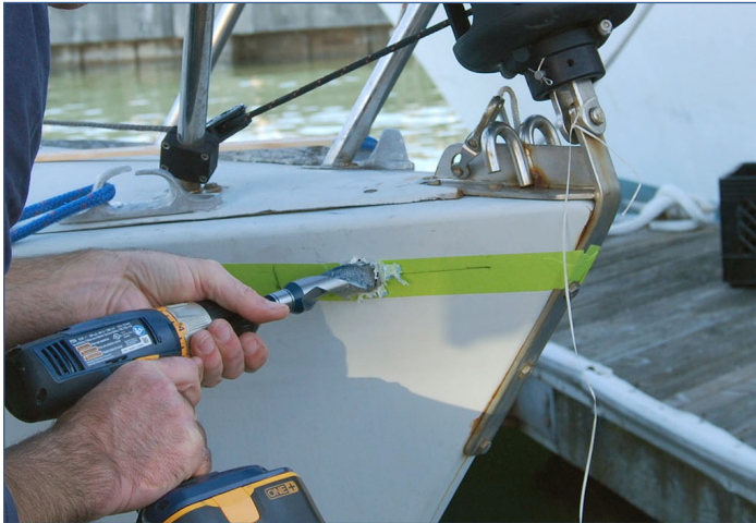
Fig 7: Drill holes using a 1" step drill.
