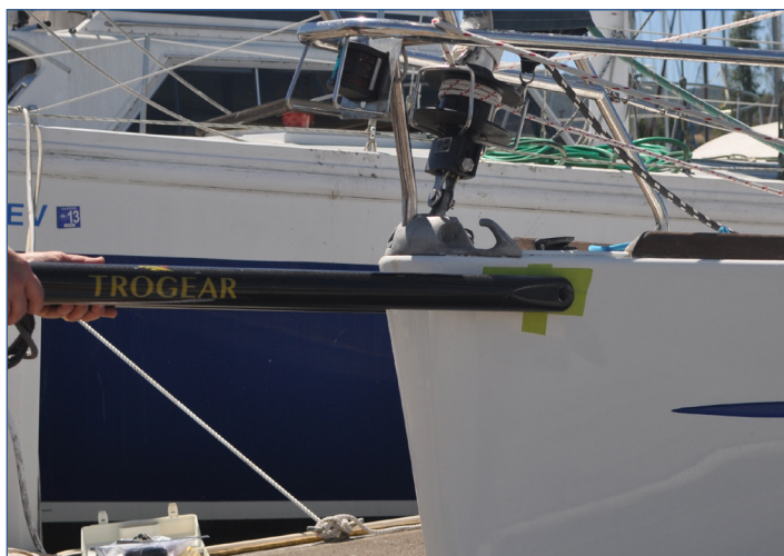
Fig 4: Use the Bowsprit to determine placement.
