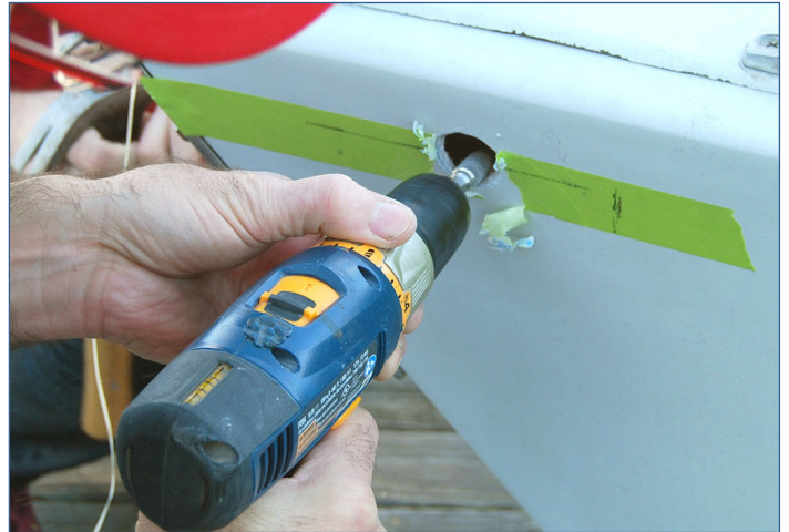
Fig 8: fine tune holes with a rotary or round file.
