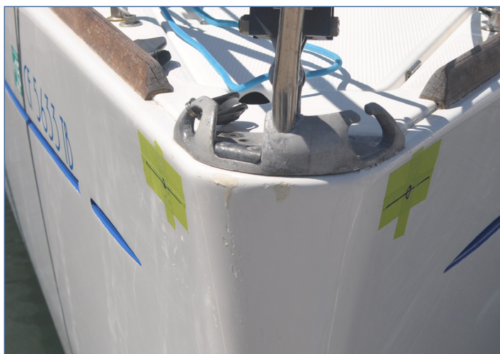
Fig 5: Using non-stretching line attached to the headstay, or other method as appropriate, check that the distances you marked are the same on each side of the boat.
