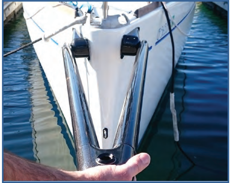
Fig. 1: Place bowsprit with mounts attached on the hull to determine location
