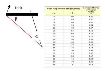
Following is one of the methods used to calculate the bobstay load:
